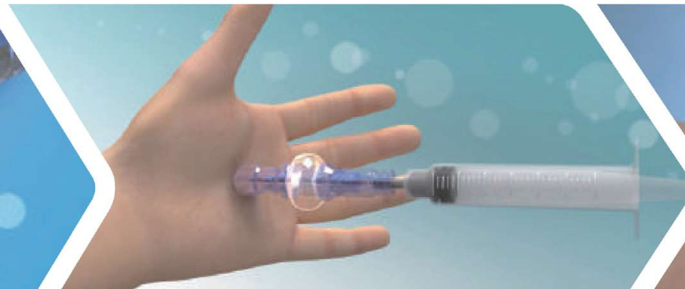
2 Execute Manual Leakage Test
